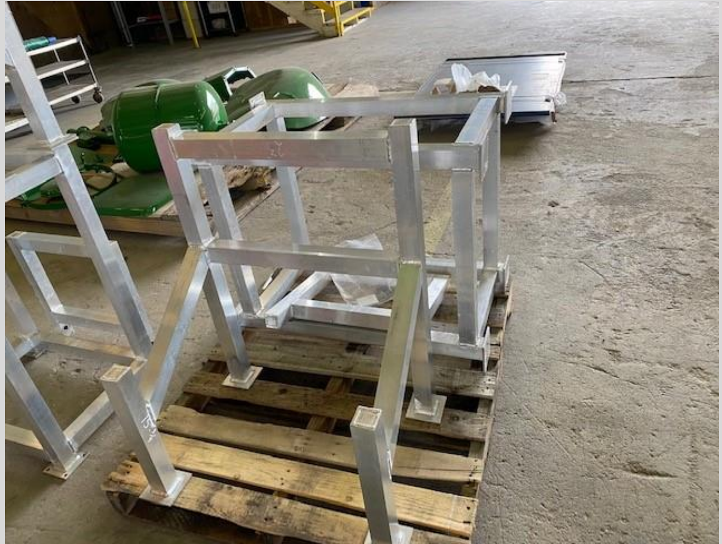
Life Raft Cradle and Stacking Frames – Fabricated awaiting anodizing before final assembly
