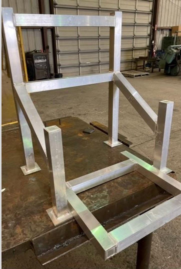
Life Raft Cradle and Stacking Frames – Fabricated awaiting anodizing before final assembly
